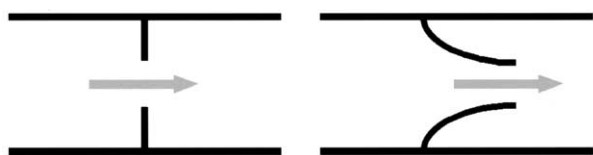
Figure 2 Schematic representation of flat sharp-edged and funnel-shaped orifices used for this in vitro study.
